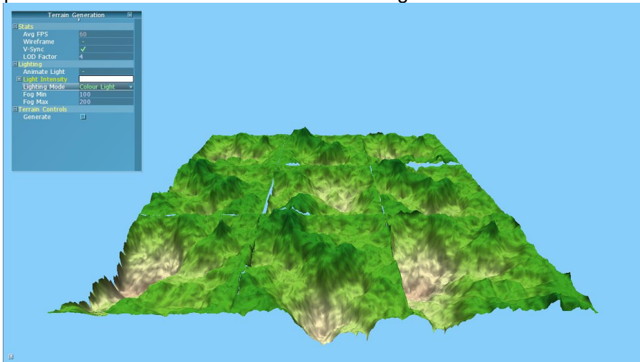
Figure 23 - Multiple blocks rendered, cracks showing where edges don't meet
